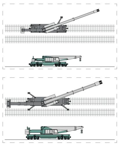
The articulated counterweight system moves the counterweight in the same angle as the boom, albeit in the opposite direction. This results in a track parallel movement of the counterweight. With a slim counterweight the counterweight will also stay clear of the adjacent line. The articulated counterweight system is also available for cranes with more than 2000 MT capacity. Our bigger cranes can lift 6-axle locomotives ahead of the coupler.
