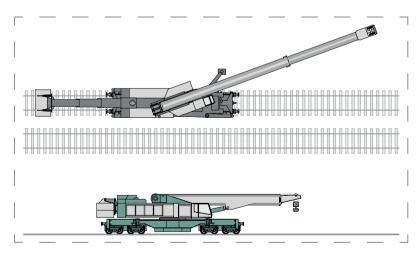
For even more operational flexibility the L-Size Crane models can be equipped with a double slewing system. This allows the boom to swivel while the counterweight remains in track direction, thus the counterweight does not interfere with the adjacent line and stays clear of tunnel walls, objects in stations or side walls of cuttings. With the counterweight in track direction only one prop needs to be set in most load cases. This makes crane work safer and more efficient.
