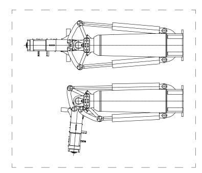
Unloading: Slag pot tipping at slag yard Tipping up to 180° by using an additional tipping device
