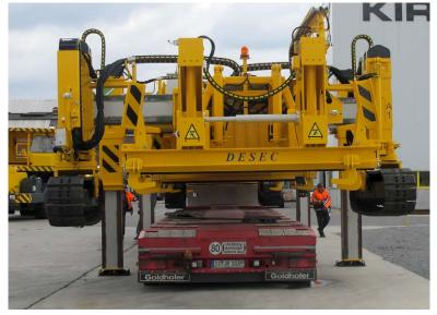
Loading onto a railroad wagon or a standard road trailer is quick and uncomplicated without the need for additional lifting equipment.
