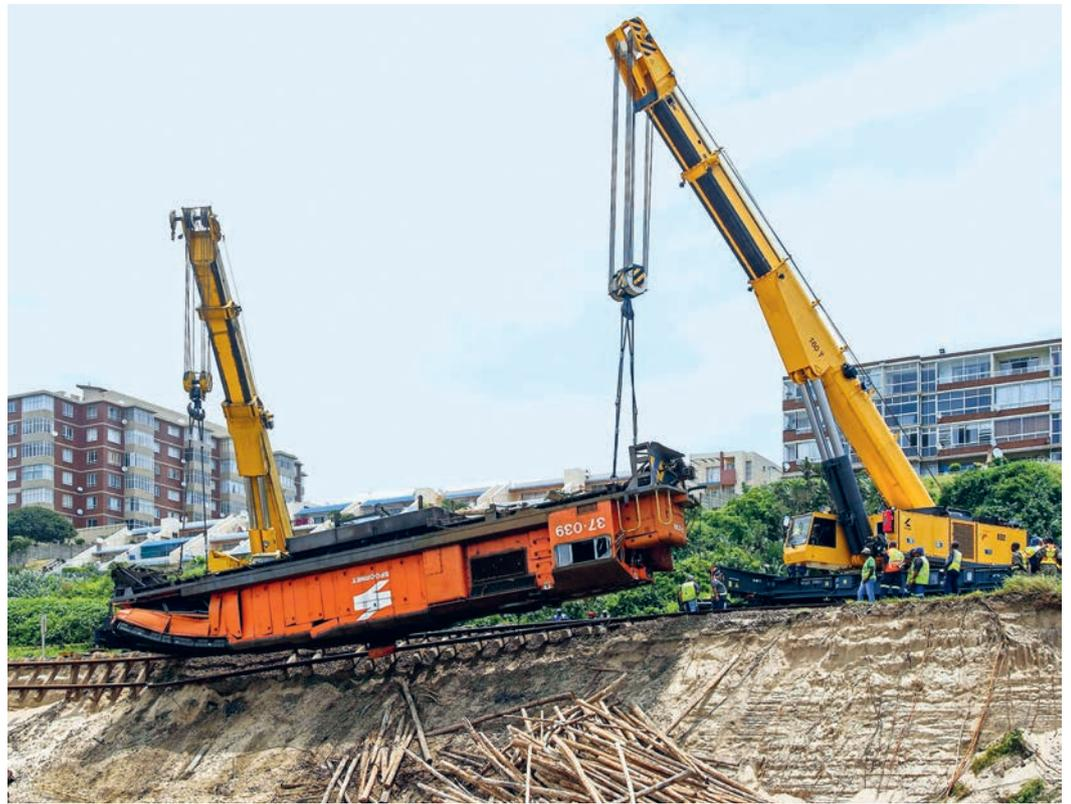
The railway crane can recover rolling stock very carefully so that it can be restored, without having to be destroyed and scrapped. This is also a significant factor for sustainability!
