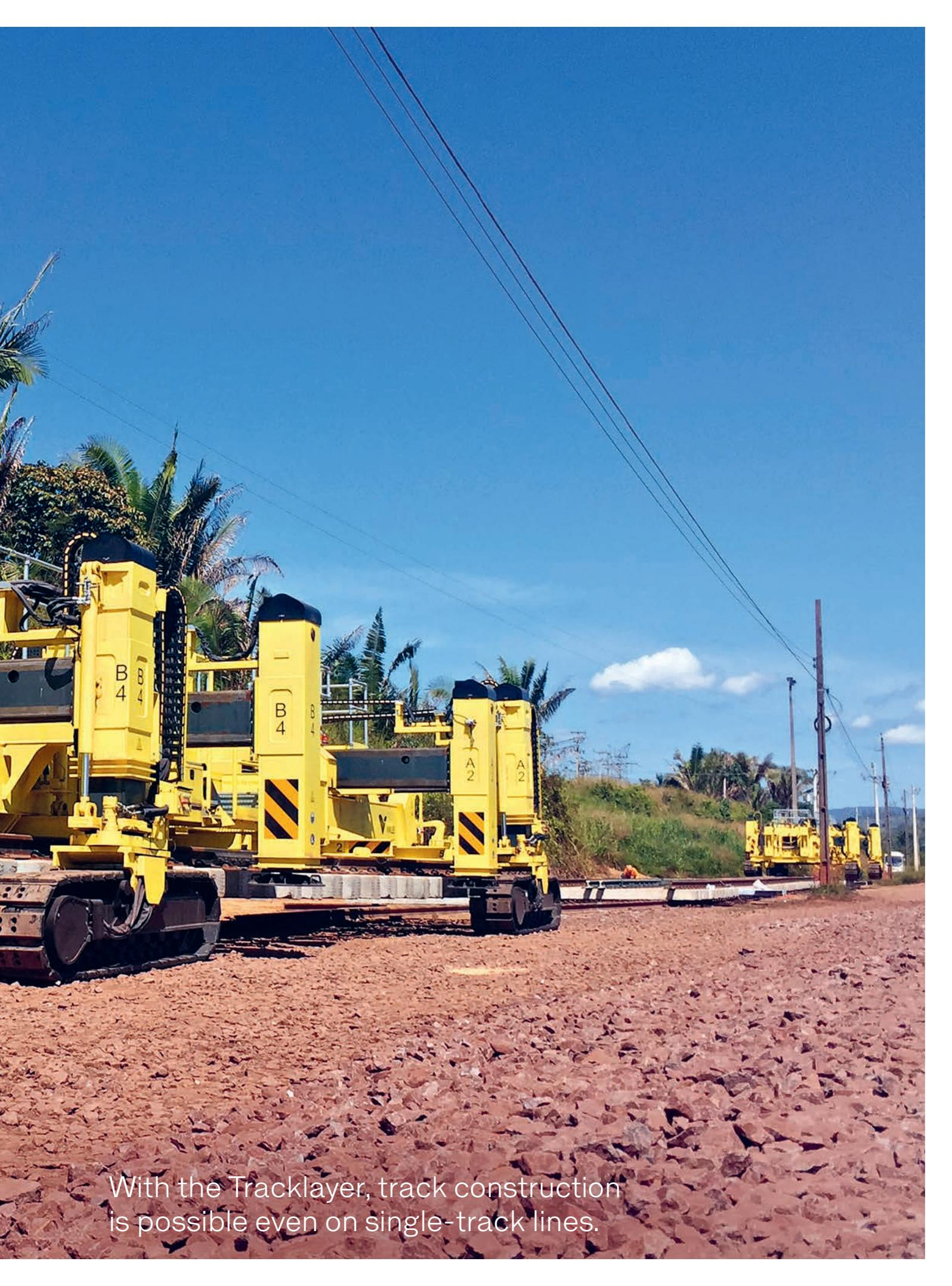
With the Tracklayer, track construction is possible even on single-track lines.
