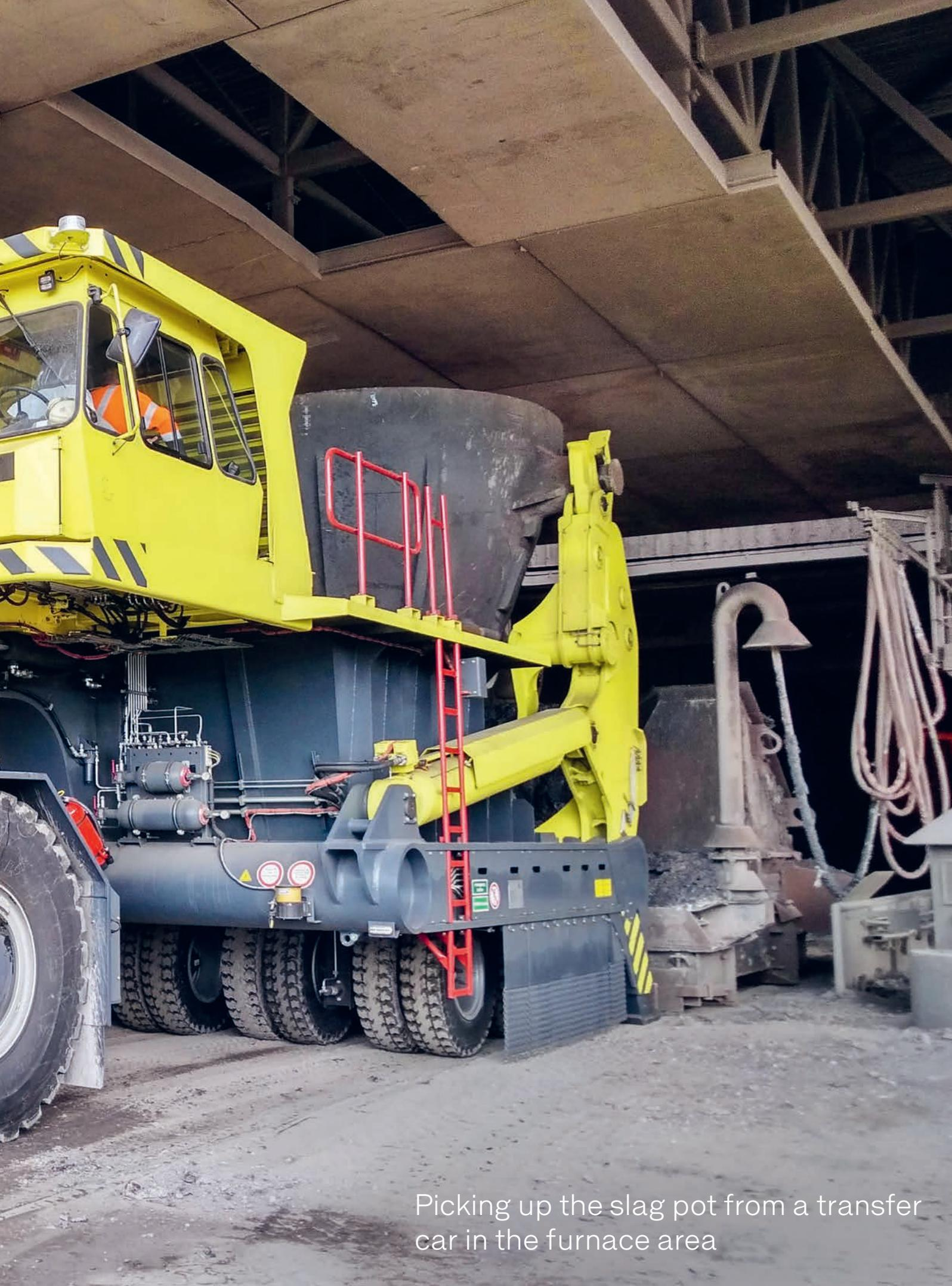
Picking up the slag pot from a transfer car in the furnace area
