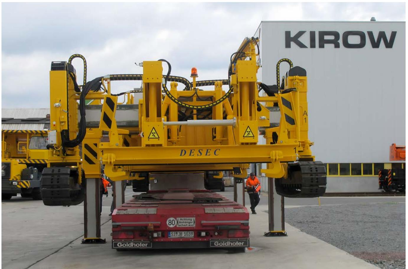
The Tracklayer can be transported by rail or road. It can load and unload itself independently without external lifting equipment on a flat rail car or truck trailer.
