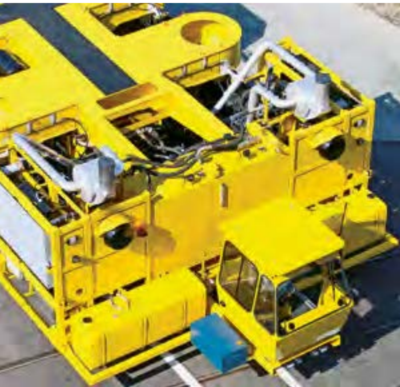
Antriebsaggregat in redundanter Ausführung / Prime mover with redundant power pack
