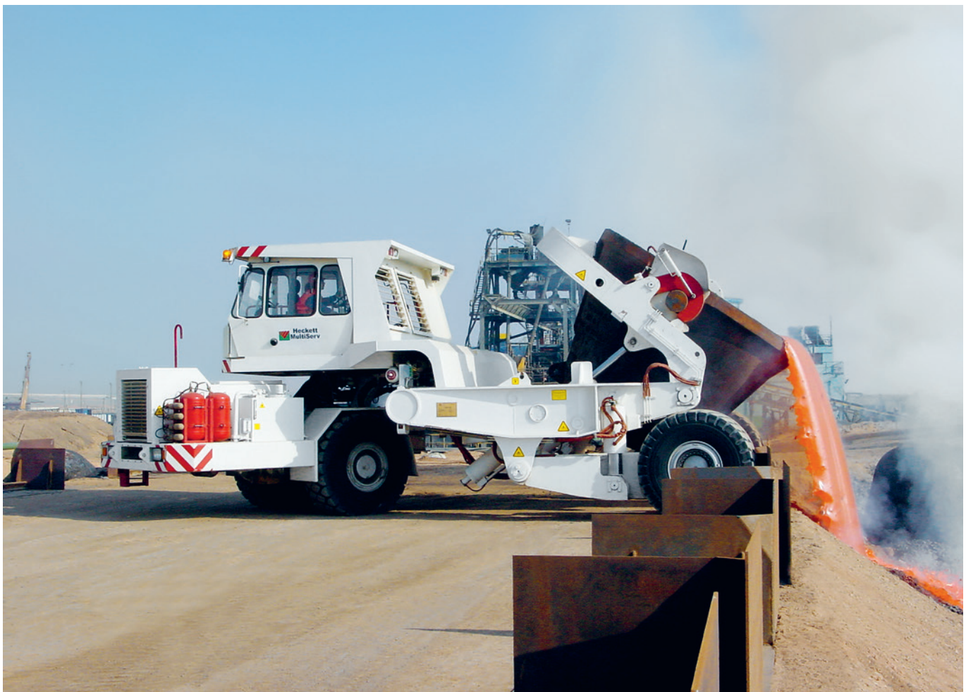
SLAG TAURUS U 60 an der Kippstation SLAG TAURUS U 60 at the tipping station
